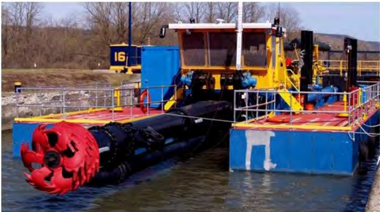
Figure 3. Photograph of a small hydraulic dredge and its barge with the machinery that powers the hydraulic dredge. The cutterhead is the red object at left.
