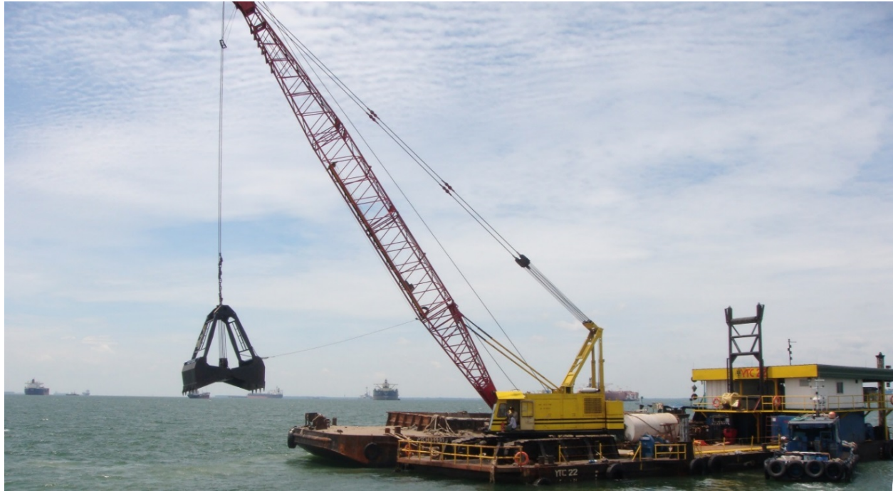
Figure 3. Barge-mounted crane dredge with clamshell bucket and a sediment transport barge tied alongside.
