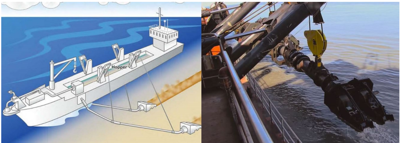
Figure 6. A drawing of a hopper dredge with its drag arms deployed is shown on the left. A retracted drag arm is shown on the right.
