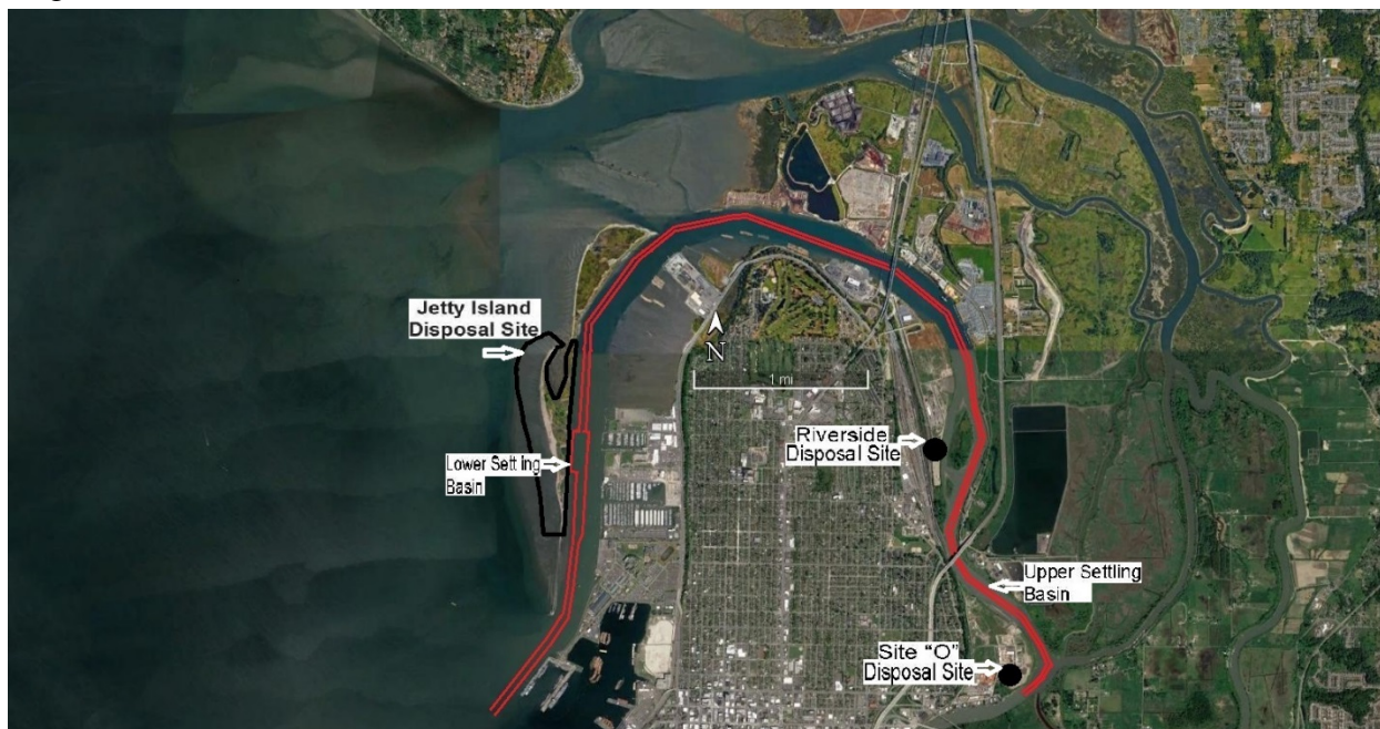
Figure 15. Everett Harbor and Snohomish River Navigation Channel. The channel and settling basins are outlined in red (Based on Figures 10 and 20 in COE 2016a).
