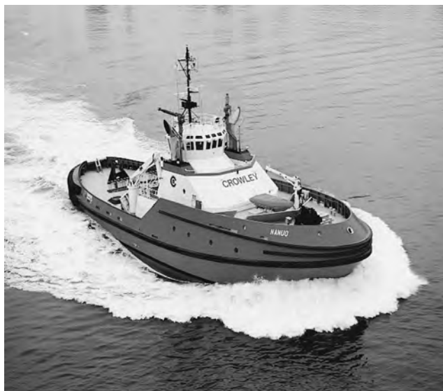
Figure 7: The 153-foot, 10,000 horsepower, state-of-the-art tractor-tug Nanuq has been put in service to escort tankers through Valdez Narrows.
