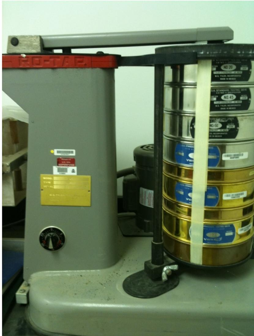
Photo 9 – Sieve analysis on Ro-Tap Model RX-29 device
