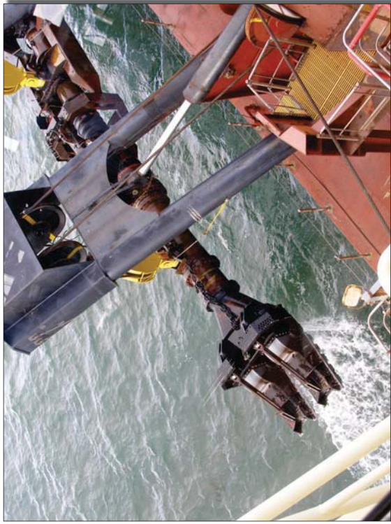
Aerial view of hopper dredge drag arm.
