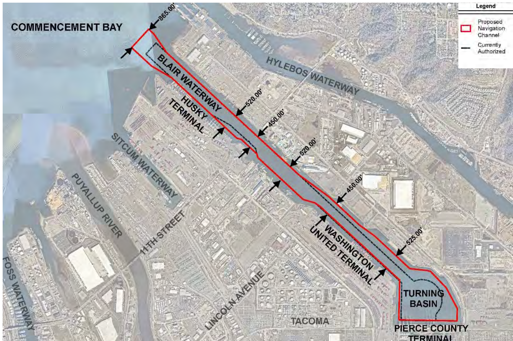
Figure 6. Tentatively Selected Plan (TSP) for the Tacoma Harbor Navigation Improvement Project, where the Blair Waterway would be dredged to -57 MLLW.
