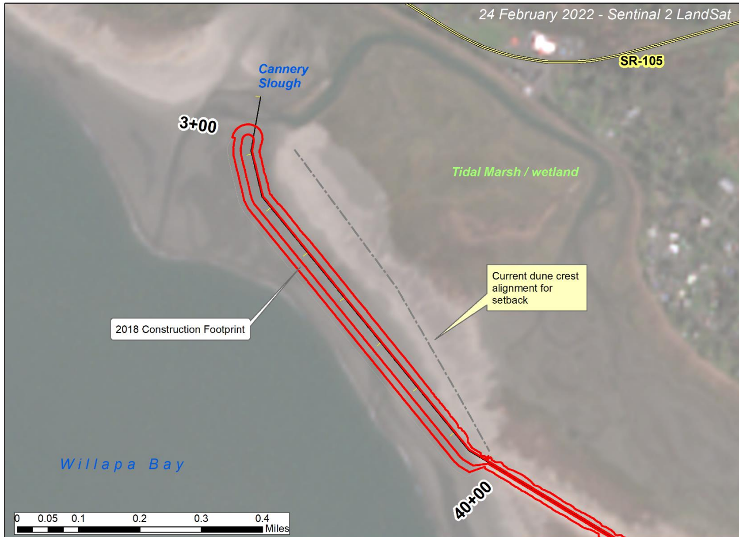
Figure A-2. Location of damaged region needing repair and approximate location setback alignment
