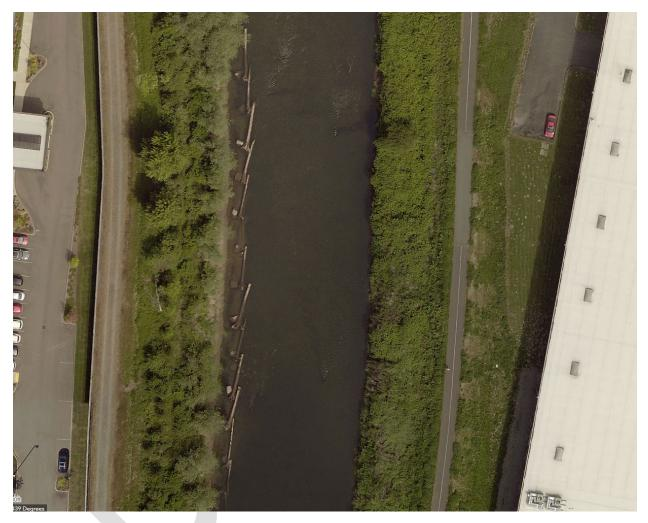
Figure A-8. Green River at RM 15.05. Desimone levee on right bank of river lacks diverse riparian vegetation and complex aquatic habitat. The left bank is a levee repair from 2008 that included aquatic habitat features (LWM). Image source: King County Orthogonal Base Imagery (2019):
