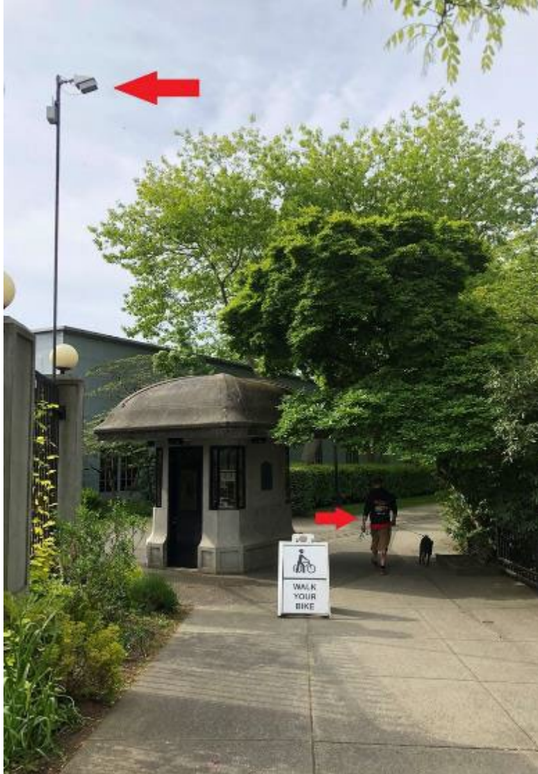
Figure 20. LiDAR pedestrian counter (top red arrow) at northeast entrance of the Locks.
