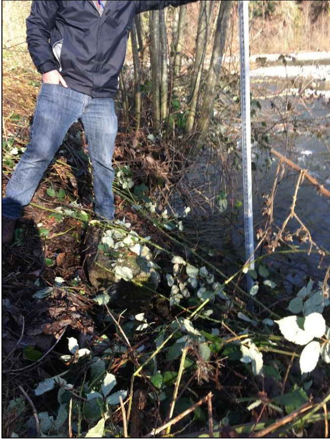
Photo 6. Bridge Street, levee measurements at Bridge Street show approximately 7 feet high repair is required.
