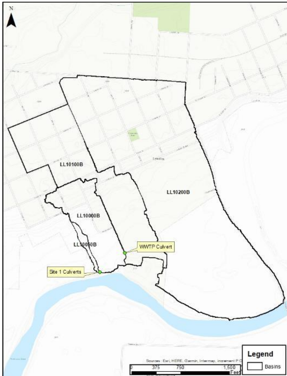
Figure 3. Culvert basin. Under normal conditions, runoff from the city of Lynden drains through the culverts at Site 1 into the Nooksack River. Access to the WWTP is via a road over the WWTP culvert, which overtops during some flood events, blocking access.
