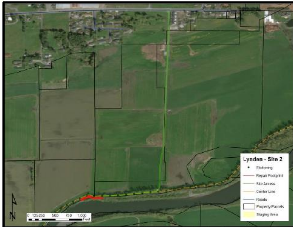
Figure 3. Aerial showing Lynden levee, repair site 2, access road and staging area.
