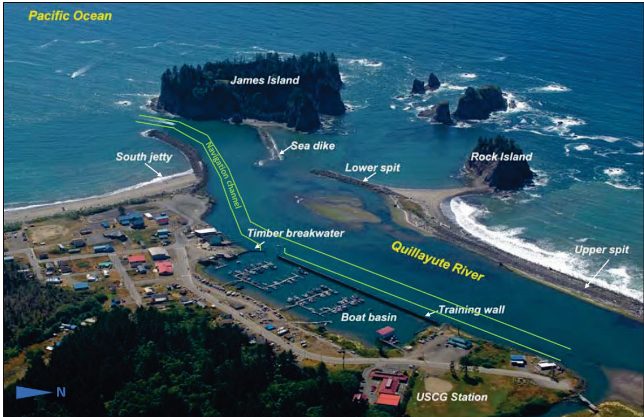
Figure 1. Federally authorized navigation features at the Quillayute River estuary, La Push, Washington. Approximate location of the navigation channel is indicated by the green lines.
