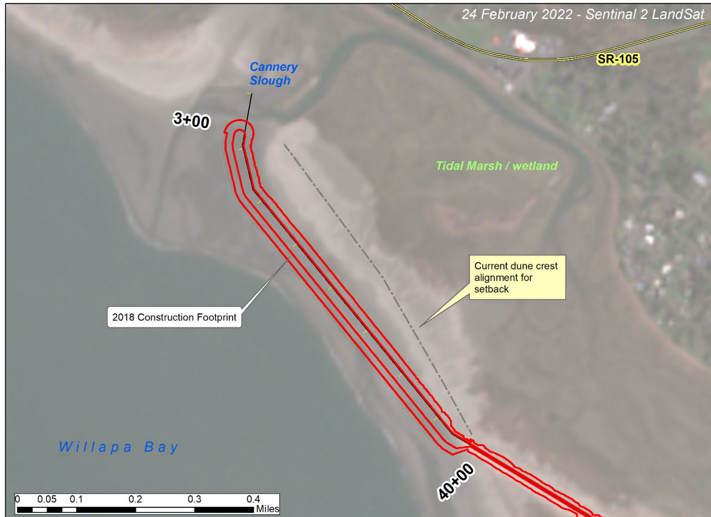
Figure 4. Location of damaged region needing repair and approximate location of setback alignment.
