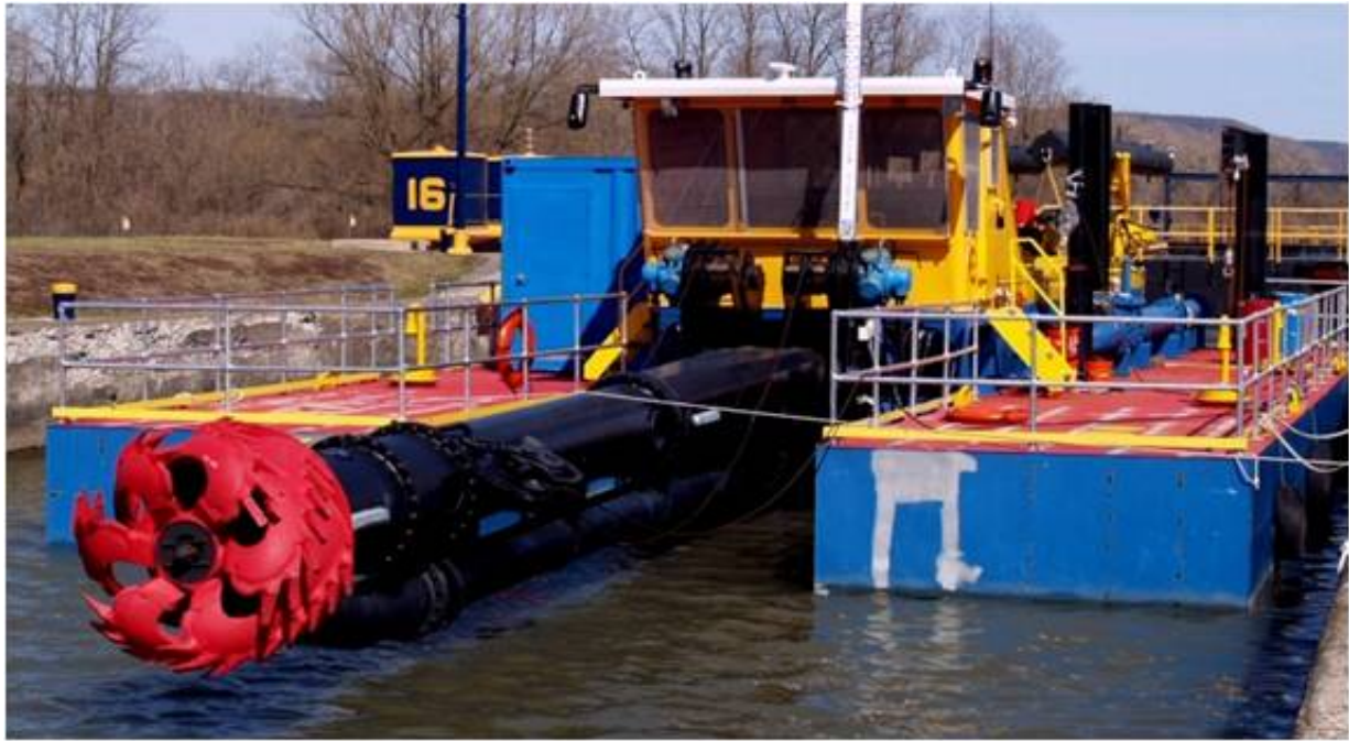
Figure 6. Small Hydraulic Dredge, Barge, and Machinery that Powers the Hydraulic Dredge
