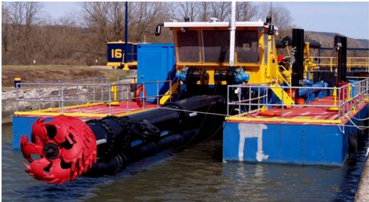
Figure 5. Small Hydraulic Dredge, Barge, and Machinery that Powers the Hydraulic Dredge
