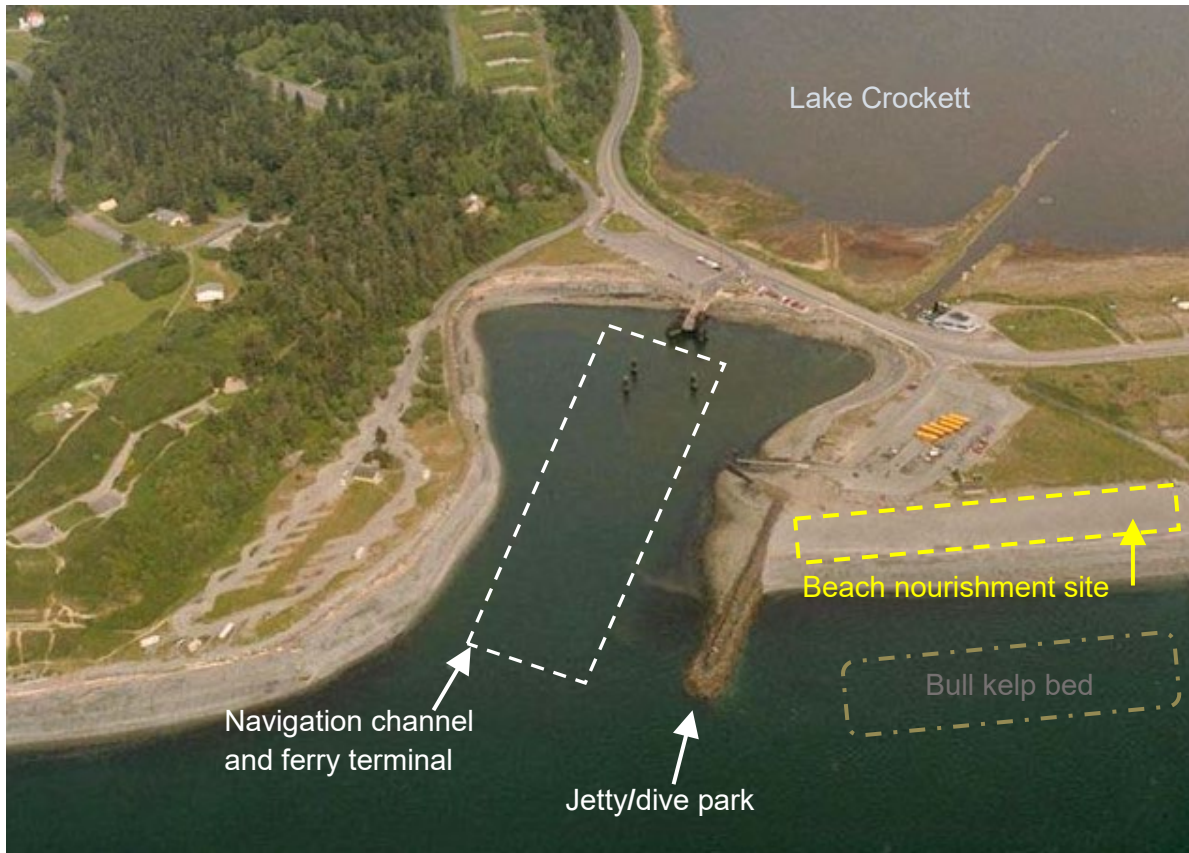
Figure 2. Aerial photograph of Keystone Harbor taken 5 May 1993 (photo courtesy of the Washington Department of Ecology).
