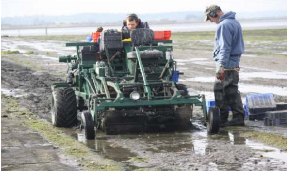
Figure 9. Mechanical clam harvester
