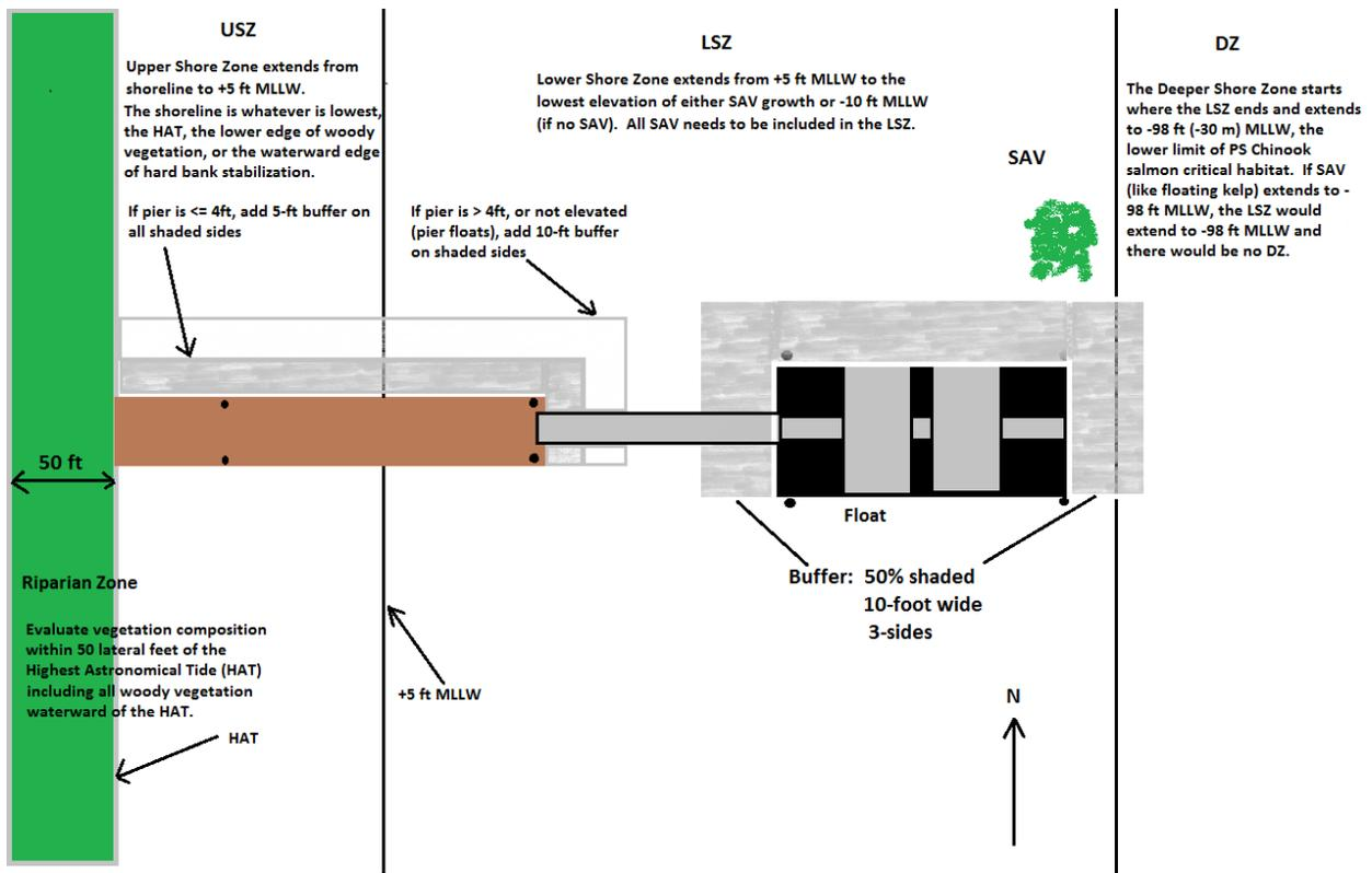
Figure 1. Conceptual depiction of different zones defined for the NHV model and a typical pier-ramp-float.
