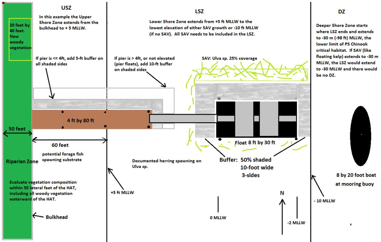
Figure 2: Example Pier Ramp and Float
